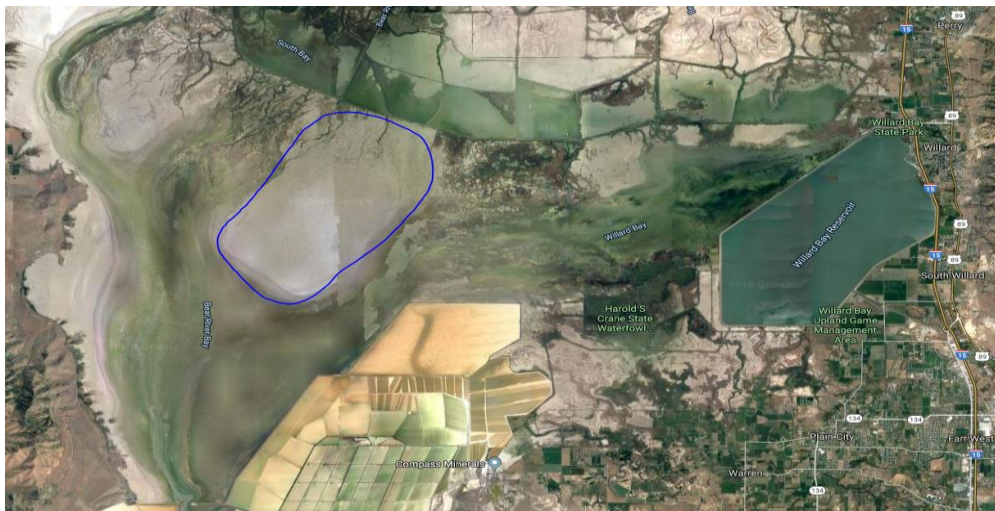
Figure 2. This photograph shows the view from satellite imagery of Willard Spur and the surrounding areas. The area circled in blue is the sandbar that appears when GSL elevations fall below 4201.9.
