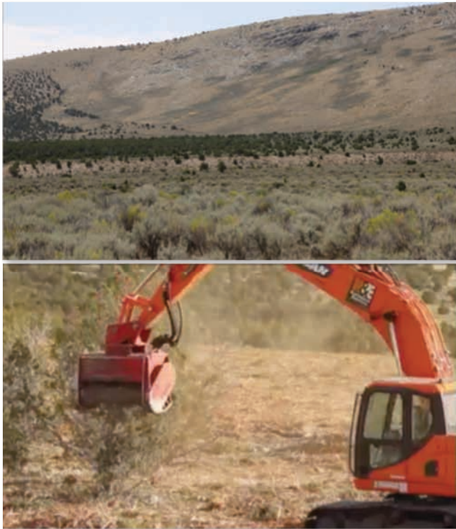
Figure 5 - Higher density encroachment areas can be managed using brush hog treatment methodology.
