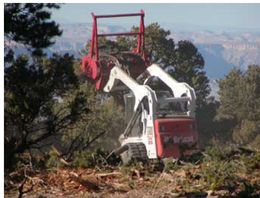
DWR personnel use a bullhog to improve wildlife habitat on the Henry Mountains.
